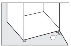
■ Also unscrew support ① from the bearing block, to level the appliance door.
